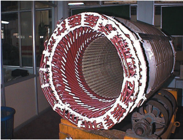
Fig 4 : Typical Wound Stator
