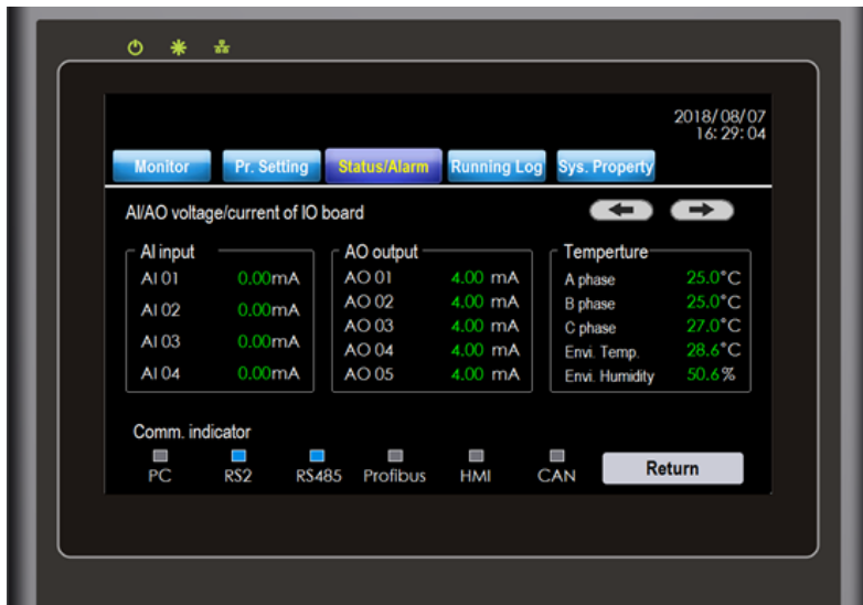
Figure 5-23 Display of AI/AO, temperature, and communication status
