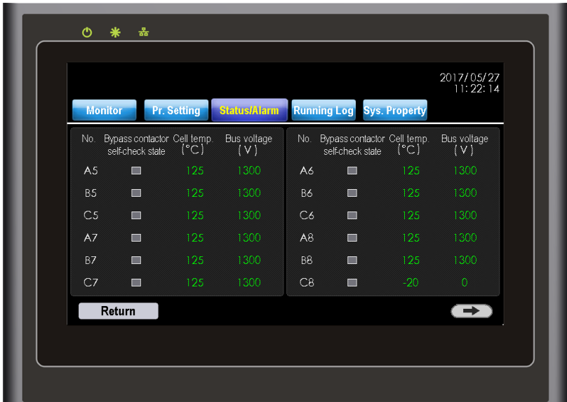
Figure 5-18 Viewing the auxiliary state of power cells
