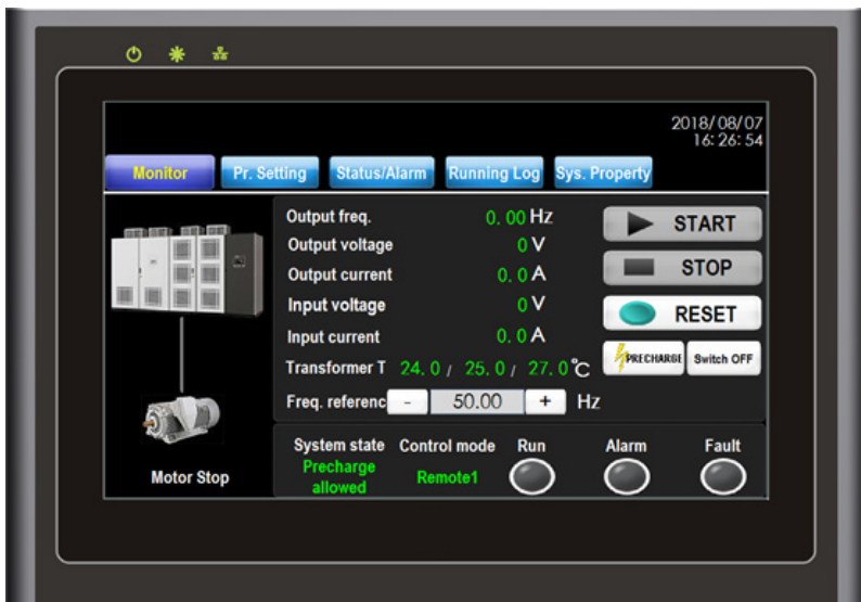
Figure 5-2 System main interface-monitor interface
