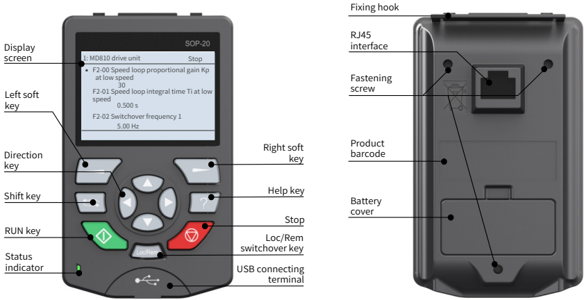
Figure 4-3 Appearance of external LCD operating panel
