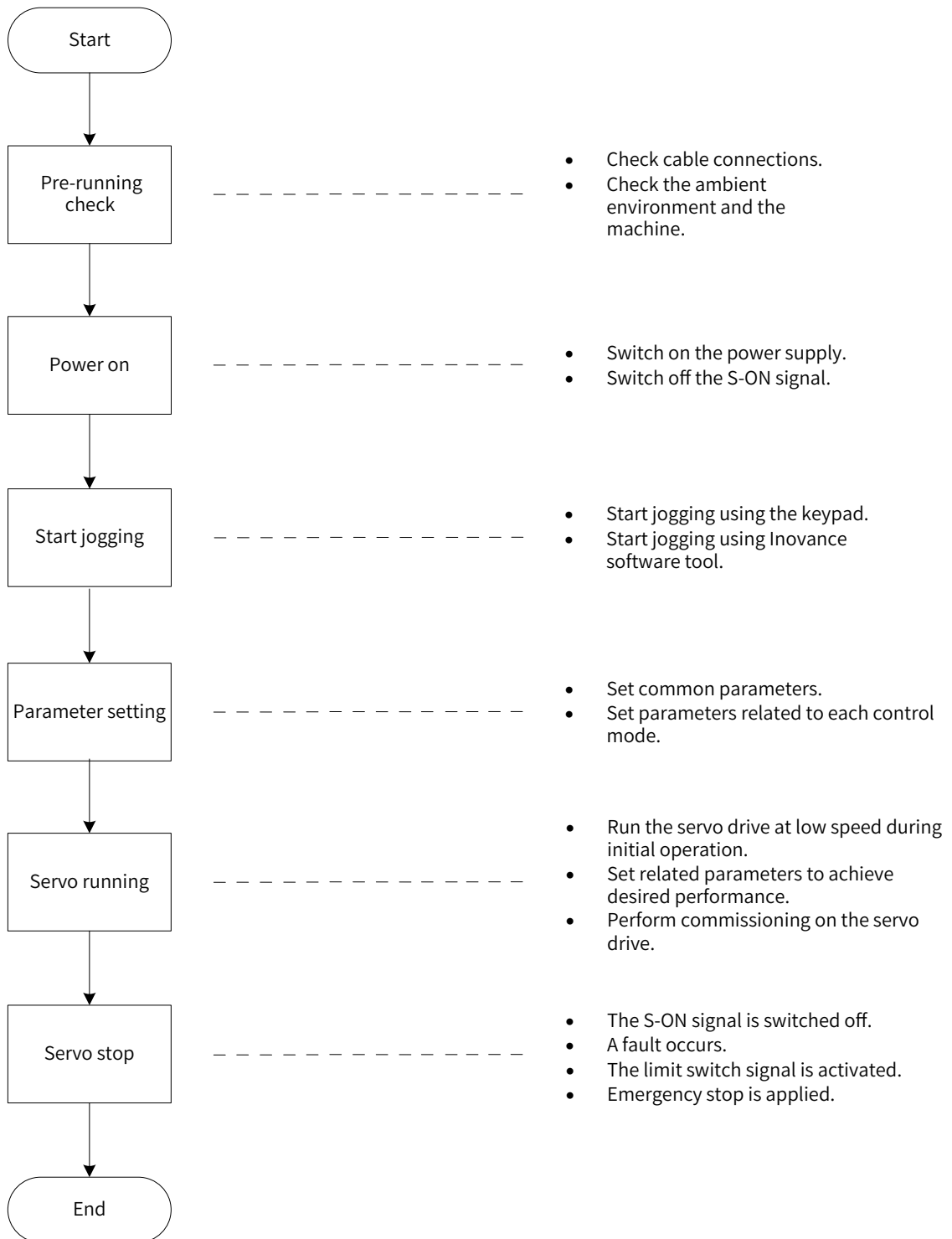
Figure 5-1 Flowchart for setting the servo drive
