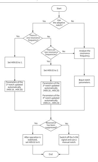
Figure 3-15 Procedure for setting the notch
