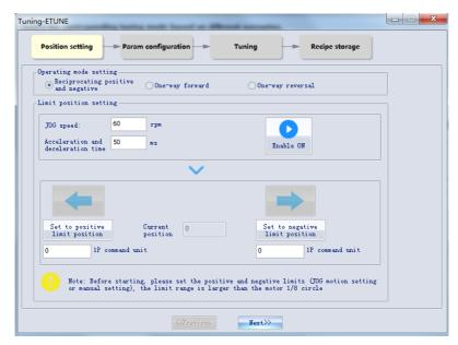
3. Designate the positive and negative limit positions allowed by the motor. The difference between the positive and negative limits defines the position reference pulses for the motor, which is also the value before multiplication/ division by the electronic gear ratio.
