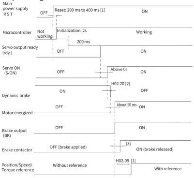
Figure 2-10 Power-on sequence diagram
