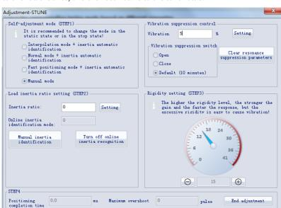
In STune mode 6, determine the minimum H08.43 (Model gain), set H09.00 to 0 for all the axes, and then set H08.43 to the save value.
