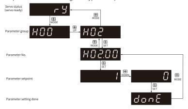
Figure 1-5 Example of parameter setting
