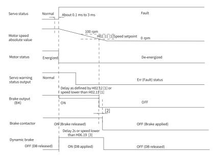
Figure 2-12 Sequence of "Dynamic braking stop, keeping de-energized state" at No. 1 fault
