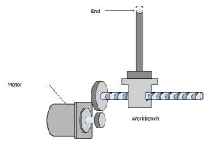
Figure 3-17 Low-frequency vibration at the mechanical end
