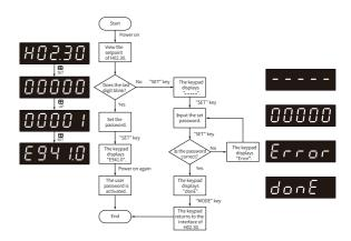
Figure 1-15 Procedure for setting the user password
