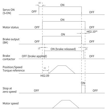
Figure 2-5 Brake sequence for motor at standstill
