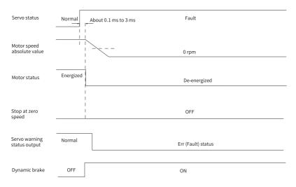
Figure 2-17 Sequence of "Dynamic braking stop, keeping dynamic braking state" at No. 2 fault (without brake)
