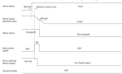
• No. 2 fault (without brake): Stop at zero speed, keeping de-energized status
