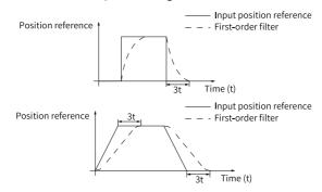
This function does not affect the displacement value (position reference sum). An excessively high setpoint delays the responsiveness, so set a proper filter time constant based on actual conditions.
