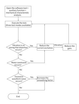
Figure 3-20 Operating procedure for mechanical characteristic analysis
