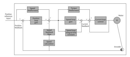
Figure 3-7 Basic control for manual gain tuning
