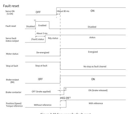
Figure 2-22 Sequence for fault reset
