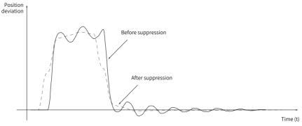
Figure 3-19 Low-frequency resonance suppression effect
