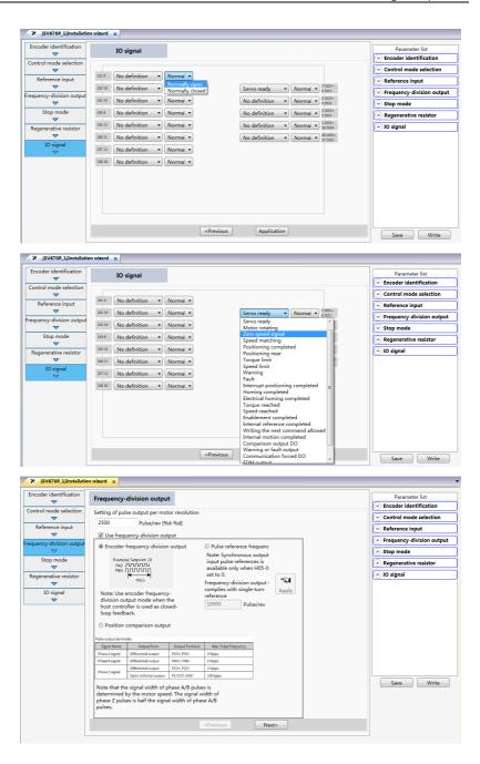
After preceding steps are done, you can view all the configured parameters in **Parameter list**. If parameters in the sub-process need to be adjusted, click the corresponding table to enter the sub-process directly and reset parameters.
