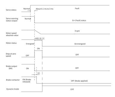
Figure 2-19 Sequence of "Stop at zero speed, keeping dynamic braking state" at No. 2 fault (with brake)
