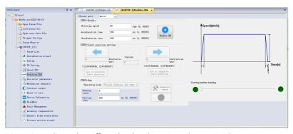
• Gain tuning: Adjusts the stiffness level and monitors the motion data.
