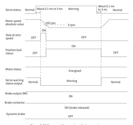
Figure 2-20 Sequence for warnings that cause stop
