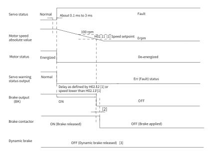
Figure 2-11 Sequence of "Coast to stop, keeping de-energized status" at No. 1 fault
