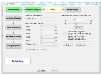
6. During gain auto-tuning, if you modify the Response fine-tuning coefficient and click "Update", gain auto-tuning will be continued based on the fine-tuning coefficient entered. After gain auto-tuning is completed, you can click "Completi..." to save parameters to EEPROM and export parameters as a recipe file.
