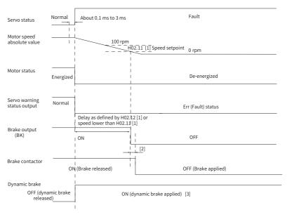
Figure 2-13 Sequence of "Dynamic braking stop, keeping dynamic braking state" at No.
