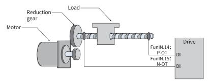
Figure 2-23 Installation of limit switches
