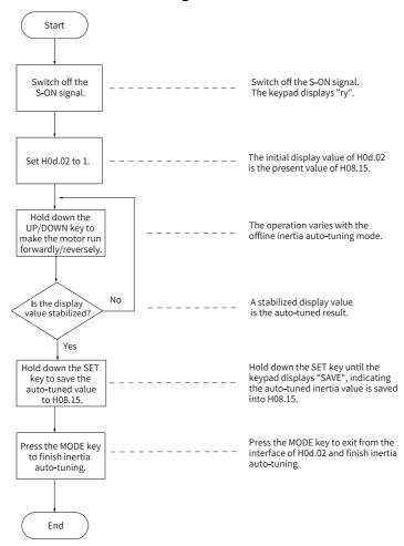
Figure 3-3 Offline inertia auto-tuning flowchart
