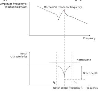
Figure 3-14 Operating principle of the notch
