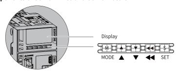
Figure 1-1 Magnified view of the keypad
