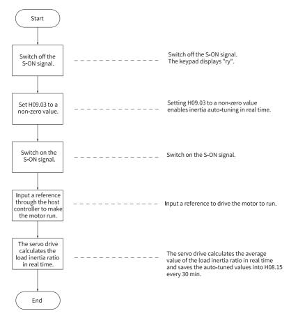
Figure 3-4 Online inertia auto-tuning flowchart
