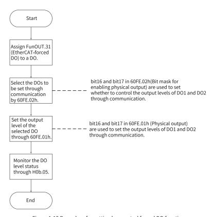
Figure 1-13 Procedure for setting bus control forced DO function
