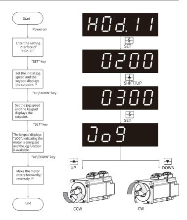
Figure 2-2 Procedure for setting the jog function
