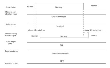
Figure 2-21 Sequence for warnings that do not cause stop
