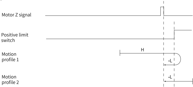
Figure 2-35 Motor running curve and speeds in Mode 8
