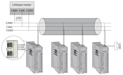
Figure 3-14 CANopen wiring diagram
