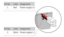
Figure 4-17 Description of the lead wire color of the battery box
