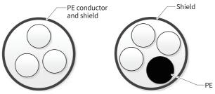
Figure 3-6 Recommended power cables
