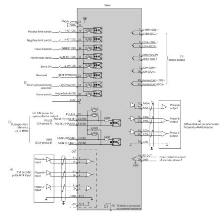
Figure 2-1 Wiring diagram of the Position Control Mode
