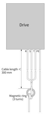
Figure 6-1 Magnetic ring on the input side
