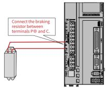
Figure 4-24 Wiring of external regenerative resistor
