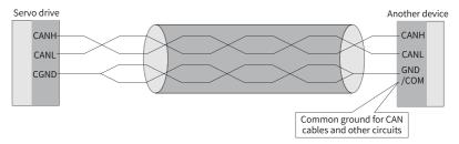
Figure 3-20 Connection mode for sharing the ground with other circuits
