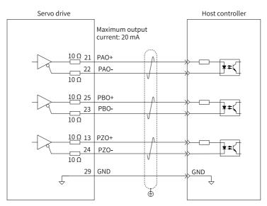
The encoder phase Z frequency-division output circuit supports open-collector signal output. Typically, this circuit provides feedback signals to the host controller in a position control system. Use an optocoupler circuit, relay circuit, or bus receiver circuit on the host controller side to receive feedback signals.
