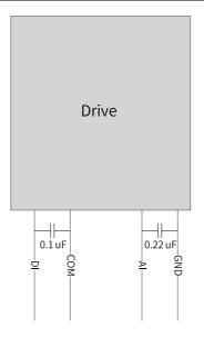
Figure 6-2 I/O signal cables with capacitance increased
