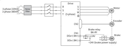
Figure 4-14 Wiring of the brake
