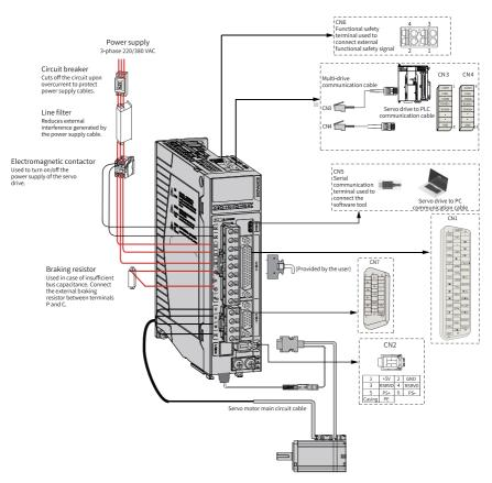
Figure 1-2 Example wiring of a three-phase 220 V or 380 V system
