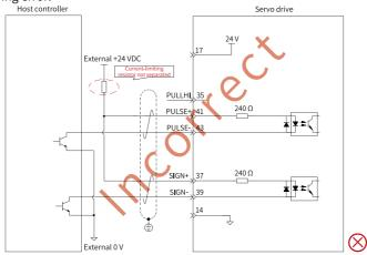
Figure 4-9 Incorrect wiring example 2: Multiple terminals share the same current lim-
