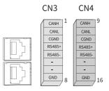
Figure 4-18 Communication Terminal pin layout of the servo drive
