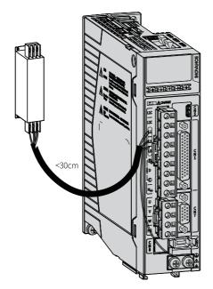
Figure 3-2 Connection of the EMC filter
