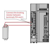
Figure 3-5 Wiring of external regenerative resistor
