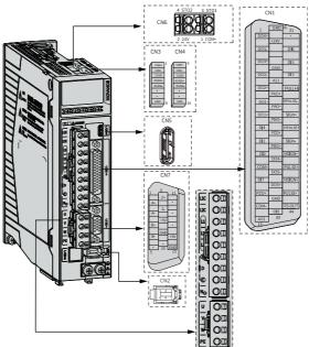
Figure 4-1 Terminal pin layout of the servo drive
