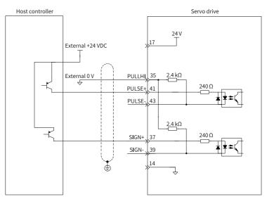
Scheme 2: Using the external resistor
