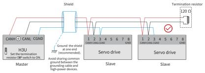
Figure 3-10 Correct CAN connection way
