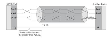
Figure 3-21 The CAN terminals of other devices have no external ground ports.
