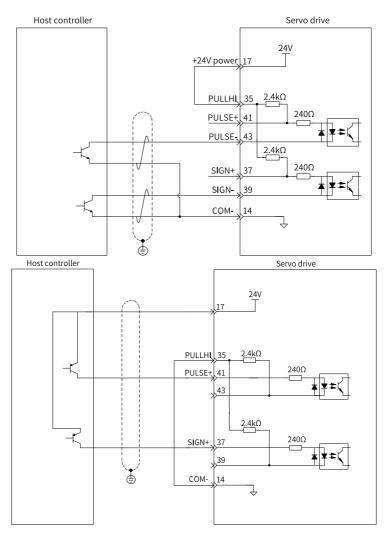
Figure 4-6 Correct: The internal 24 V power supply of the servo drive is used.
