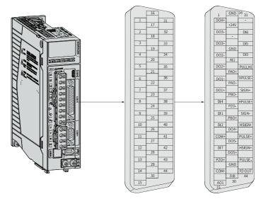
Figure 4-5 Control terminal pin layout of the servo drive
