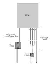
Figure 3-4 Connection of the magnetic buckle
