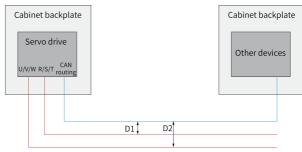
Figure 3-22 Recommended routing modes
