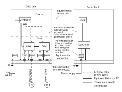
Figure 3-28 Recommended wiring for the control cabinet system
