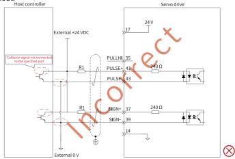
Figure 4-11 Incorrect wiring example 4: Terminals are connected incorrectly, resulting in terminal burnout.
