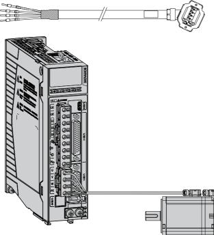
Figure 4-4 Wiring between the servo drive and terminal-type motor
