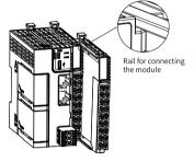
Install an DIN rail end plate to both sides of the master or module. To mount the end plate, hook the bottom of it to the bottom of the DIN rail, rotate the end plate to hook the top of it to the top of the DIN rail, and then tighten the screw to lock the end plate in place, as shown below.
