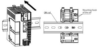
Make sure the DIN rail mounting hook of the module is locked. The locked and unlocked states of the mounting hook are shown below.
