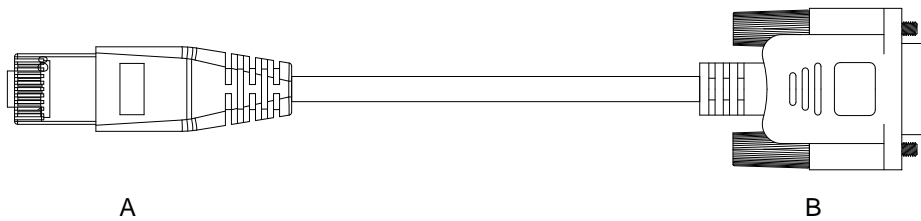
Figure 3-30 Appearance of the PC communication cable
