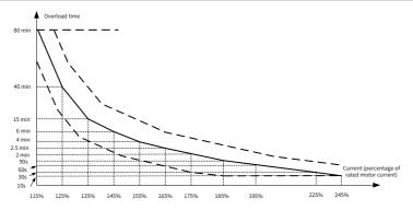
Inverse time-lag curve of motor overload protection
