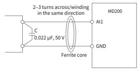
Figure 2-5 Installing a ferrite core
