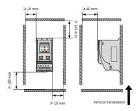
Installing a single AC drive
