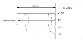
Figure 2-4 Wiring of AI terminals
