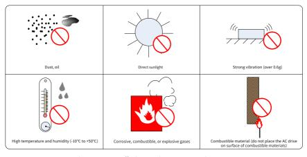
Figure 2-1 Installation environment requirements
