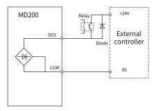
Figure 2-9 Wiring of DO terminals
