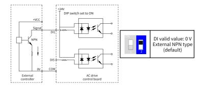
Figure 2-6 Sink wiring
