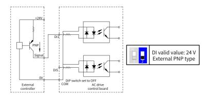
Figure 2-8 Source wiring
