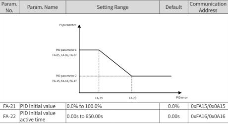
When the AC drive starts up, the PID starts closed-loop algorithm only after the PID output is fixed to the PID initial value (FA-21) and lasts the time set by FA-22.
