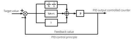
PID control principle
