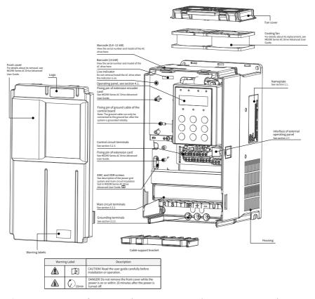
Figure 1-2 Components (MD290T0.4G/0.7PB to MD290T15G/18.5PB, MD290-2T0.4G/0.7PB to MD290-2T7.5G/11PB)
