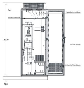
Figure 3-7 Cabinet with fans on the top
