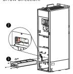
4 Loosen screws from each fan cover and remove the fans.
