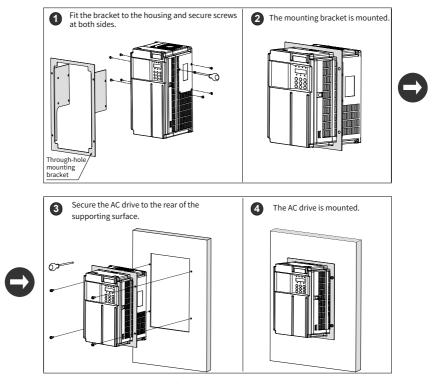
Figure 3-4 Through-hole mounting of MD290T0.4G/0.7PB to MD290T37G/45P(B) and MD290-2T0.4G/0.7PB to MD290-2T18.5G /22P(B)
