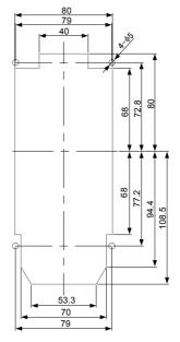
Figure 2-5 Sheet metal slot dimensions (unit: mm)
