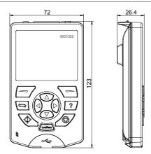
Figure 2-4 Mounting dimensions of the MDKE9 external operating panel (unit: mm)
