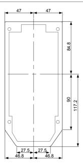
Figure 2-6 Mounting base dimension limits (unit: mm)
