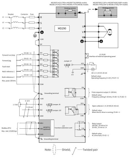
Figure 3-8 Typical wiring
