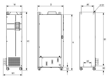
Figure 1-6 Overall and mounting dimensions of MD290T200G to MD290T450G and MD290T220P to MD290T500P
