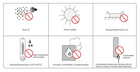
Figure 3-1 Installation environment requirements
