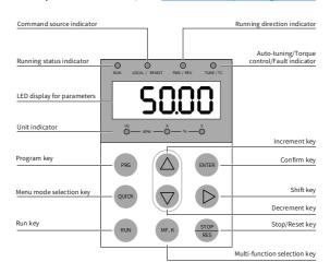
Figure 4-1 Details of the operating panel
