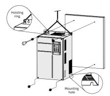
Figure 3-3 Backplate mounting of MD290T45G/55P(B) to MD290T160G/200P and MD290-2T22G/30P(B) to MD290-2T55G/75P
