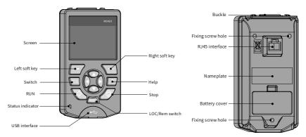
Figure 2-3 Appearance of the MDKE9 external operating panel
