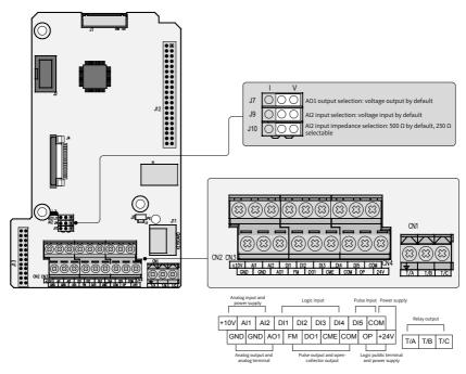
Figure 3-12 Control circuit terminal arrangement
