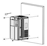
Figure 3-2 Backplate mounting of MD290T0.4G/0.7PB to MD290T37G/45P(B) and MD290-2T0.4G/0.7PB to MD290-2T18.5G/22P(B)
