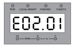
Figure 1-5 Fault code
