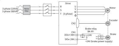
Figure 4-34 Wiring of the brake
