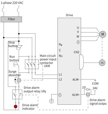
Figure 4-17 Main circuit wiring
