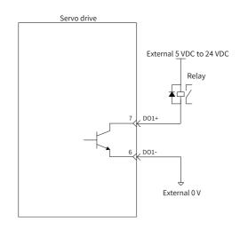
When the host controller provides relay input, a flywheel diode must be installed. Otherwise, the DO terminals may be damaged.
