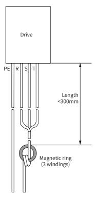
Figure 7-1 Magnetic ring on the input side
