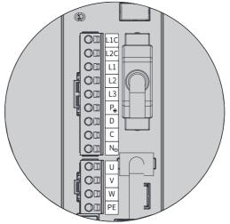
Figure 4-10 Main circuit terminal pin layout of servo drives in size C (SV660PS7R6I) and size
