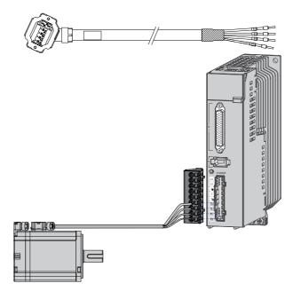
Figure 4-14 Wiring between the servo drive and terminal-type motor Table 4–15 Description of the power cable connector (motor side)
