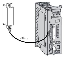
Figure 1-13 Installing the AC input reactor
