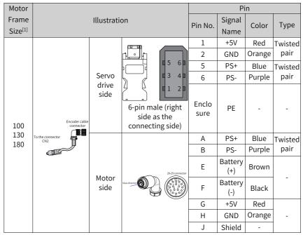
Table 4–32 Absolute encoder cable connector (MIL-DTL-5015 series 3108E20-29S aviation connector)
