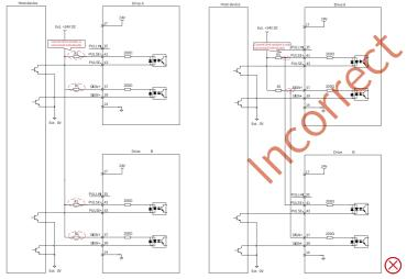
Figure 4-30 Incorrect wiring example 5: Multiple terminals share one current limiting
