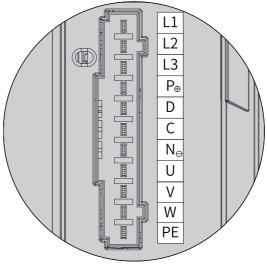
Figure 4-9 Pin assignment of main circuit terminal of servo drives in SIZE B
