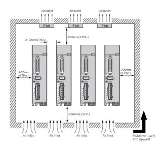
Figure 1-3 Clearance for side-by-side installation
