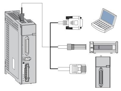
Figure 4-40 Wiring of communication cables
