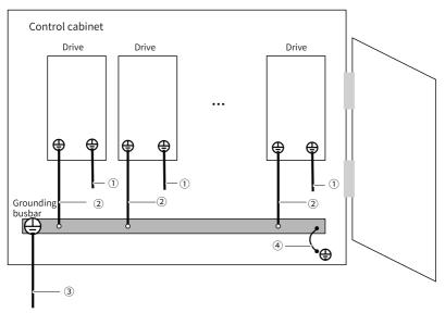
Table 4–20 Description for grounding of multiple drives installed side by side
