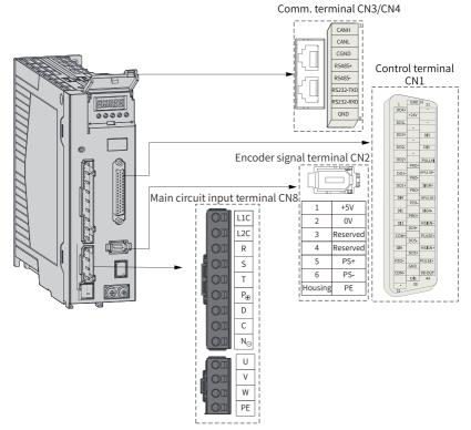
Figure 4-4 Terminal pin layout of servo drives in size C (SV660PT3R5I, SV660PT5R4I) and size D (SV660PT8R4I, SV660PT012I)
