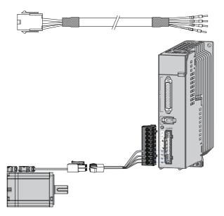
Figure 4-15 Wiring between the servo drive and terminal-type motor Table 4–16 Description of the power cable connector (motor side)
