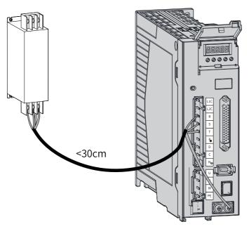
Figure 4-16 Installing the filter
