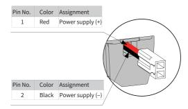
Figure 4-37 Lead wire color of the battery box
