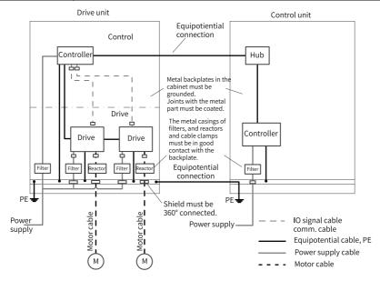
Figure 4-20 Recommended wiring for the control cabinet system
