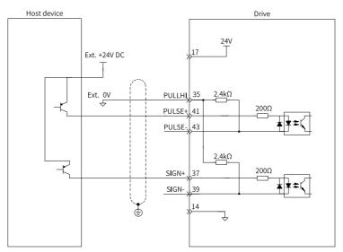
Scheme 2: Using the external resistor
