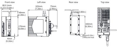
Screw: 3-M4; tightening torque: 1.2 N · m Weight: 1.8kg (3.97lb.)
