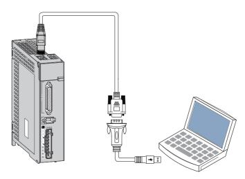
Figure 4-49 PC communication cable
