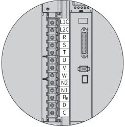
Figure 4-12 Pin assignment of main circuit terminal of servo drives in size E
