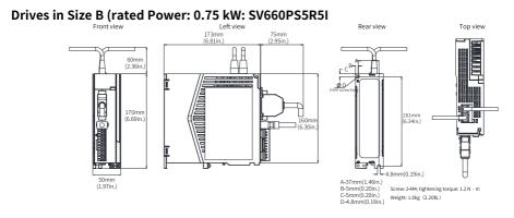
Figure 1-7 Dimension drawing of servo drives in size B
