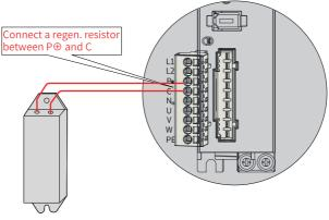
Figure 4-50 Wiring of external regenerative resistor
