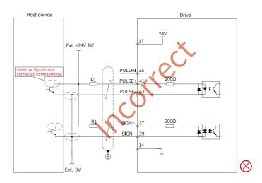
Figure 4-29 Incorrect wiring example 4: Terminals are connected incorrectly, result-
