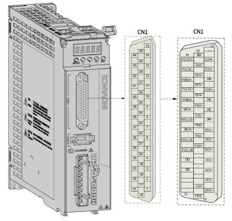
Figure 4-22 Control terminal pin layout of servo drives in sizes A and B
