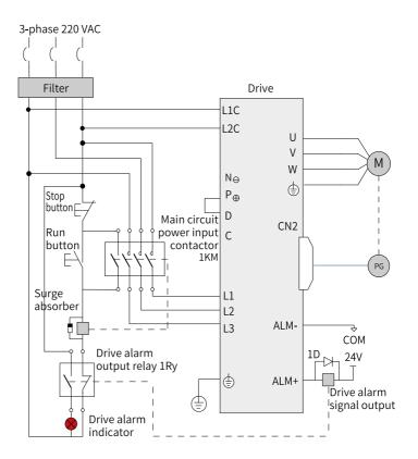
Figure 4-18 Main circuit wiring of three-phase 220 V models
