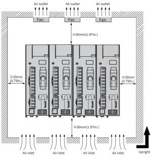
Figure 1-5 Zero-clearance installation
