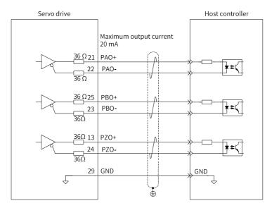
Figure 4-32 Optocoupler receiving circuit
