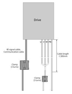
Figure 1-15 Installation of the ferrite clamp
