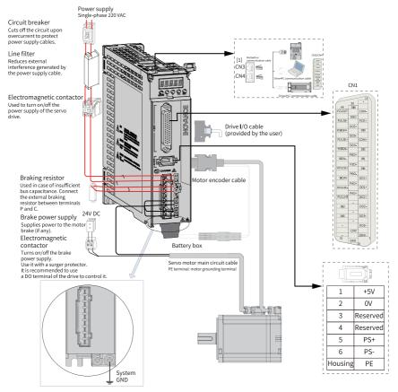
Figure 2-1 Wiring example of a single-phase 220 V system
