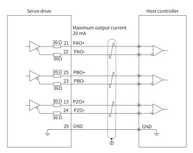
Figure 4-31 Differential receiving circuit
