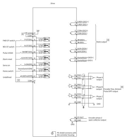
Figure 3-2 Wiring Diagram for Torque Control Mode
