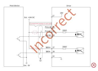
Figure 4-26 Incorrect wiring example 1: The current limiting resistor is not connected,
