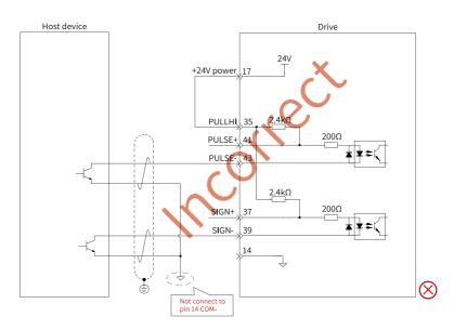
Figure 4-25 Incorrect: Pin 14 (COM–) is not connected, leading to failure in forming a closed-loop circuit.
