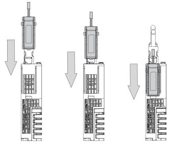
Figure 4-38 Installing the battery box (bottom view)
