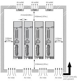
Figure 1-4 Clearance for compact installation
